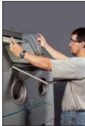
The tilt-out frame makes changing the tempered-glass window a snap.
